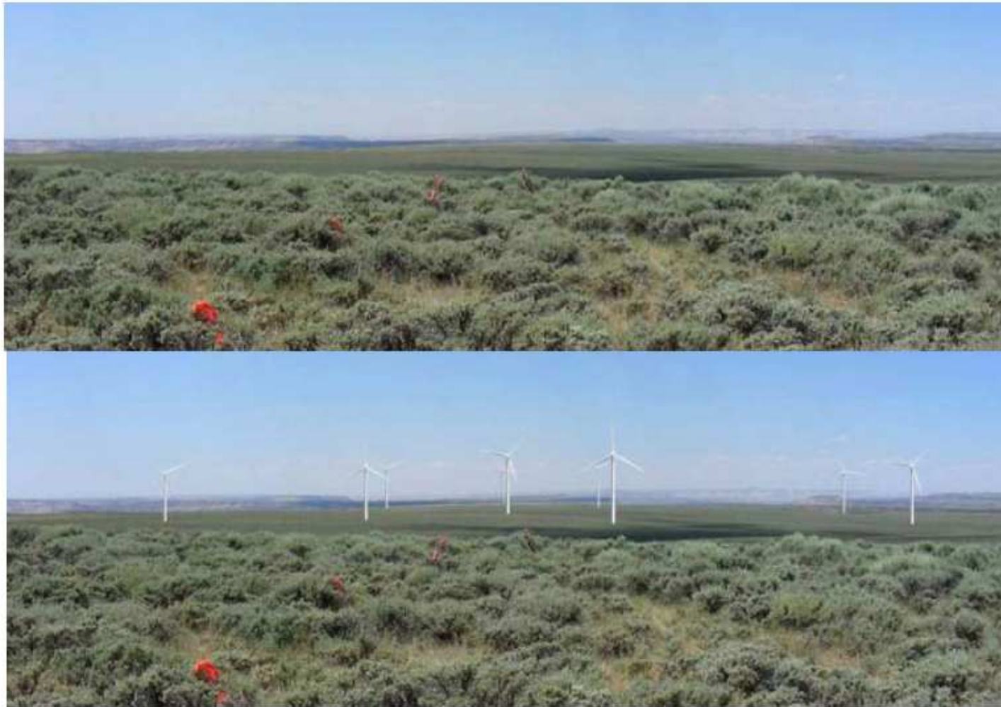
Simulation of a hypothetical wind project at a typical location in the Intermountain West. Simulated turbines are at distances of approximately 1.75 to 3 miles from the observer. Simulation courtesy of Tetra Tech EC, Inc.
